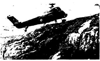
Wessex helicopter hovering with one wheel on the slope above a sea cliff on the Isle of Anglesey, North Wales, Rescue personnel exiting should move down slope to avoid rotor.
